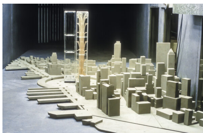
Figure 2.4 – Aerospace 1:400 scale wind tunnel models being used for the World Trade Center at the laboratories in 1965. Source: https://skyscraper.org/exhibitions/giants-twin-towers-and-the-twentieth-century/
