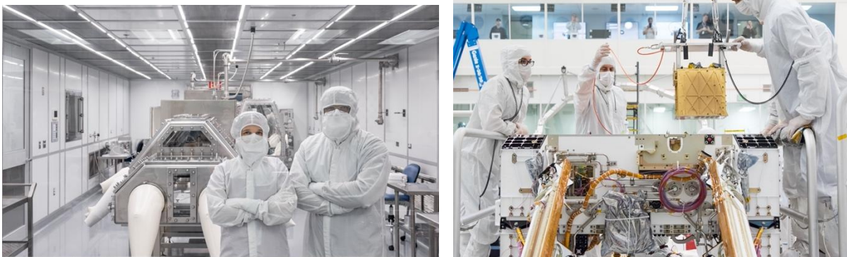
Figure 1.20 – Inside two example cleanrooms at ISO 6 and 7 standards (left and right images, respectively). Source: NASA image and video library.
