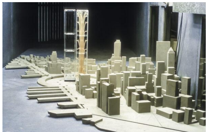
Figure 2.4 – Aerospace 1:400 scale wind tunnel models being used for the World Trade Center at the laboratories in 1965. Source: https://skyscraper.org/exhibitions/giants-twin-towers-and-the-twentieth-century/
